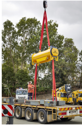
Figure 2.16: The R-Series is a commercially available load rotation device that uses gyroscopes and was launched by the Australian company Verton in 2019. (Picture by Rod Pilbeam)
