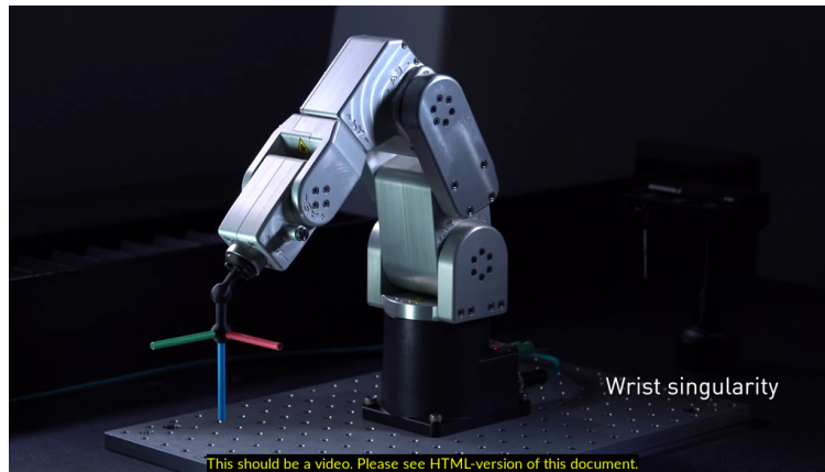
Figure 9.1: Illustration of a singularity in a six-axis industrial robot. Once the two axis are in line they can in theory rotate an infinite amount with producing a lateral movement. The speed at which they have to rotate to maintain a constant lateral motion therefore also goes to infinity. Animation by Mecademic 81
