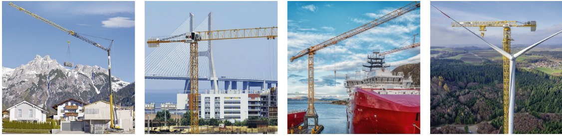
Figure 4.1: Cranes used to estimate parameter space of construction cranes. From left to right (increasing payload): L1-24, 71 EC-B, 380 EC-B, 1000 EC-B.
